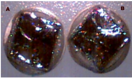
BREAKS AT SILICON DIE NO VISIBLE VOIDS.
