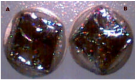
BREAKS AT SILICON DIE NO VISIBLE VOIDS.
